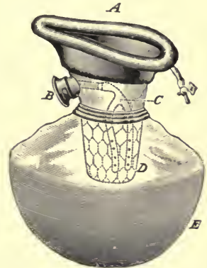
FIG. 14.—The Ormsby ether inhaler. A, face-piece with inflatable rubber edge (detachable). B, tap for admission of air and addition of ether, which passes to the cage D through the tube C. E, the rubber bag which permits re-breathing.
